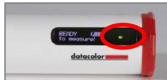
An LED indicator displays the current state of the device. See [Status LED](#) for details.
